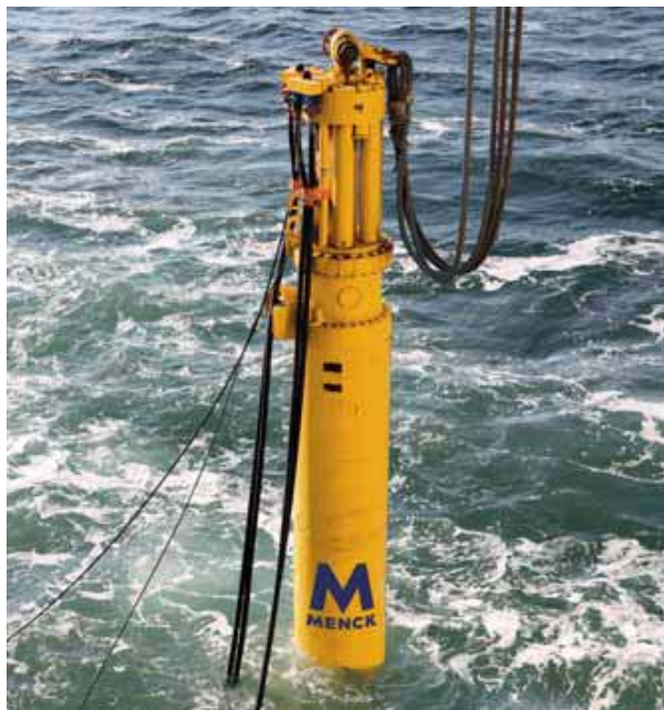
Free riding hammer for jacket installation
